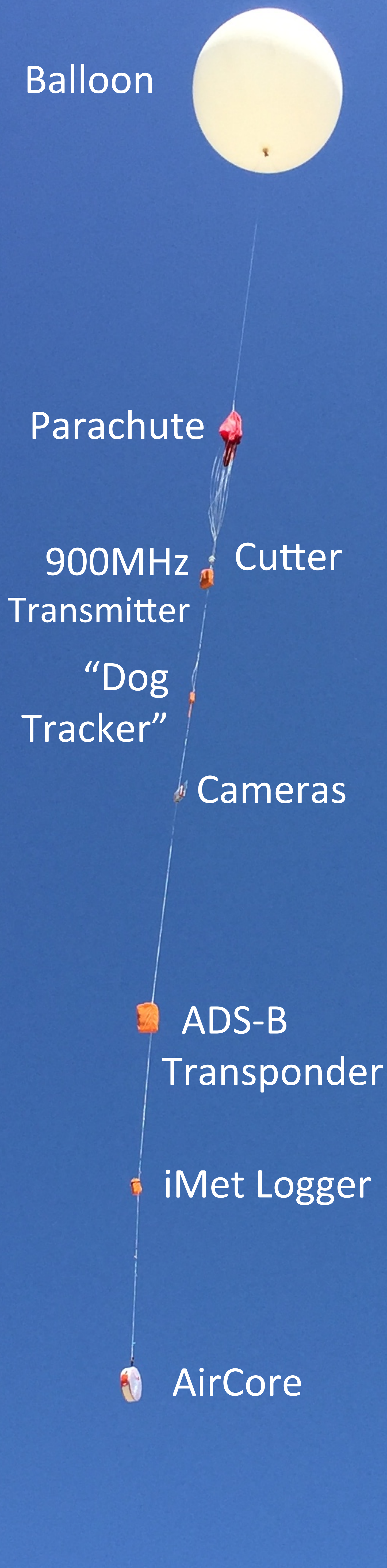
Figure 2. Current AirCore design, with 100 m 1/8" SS coil
